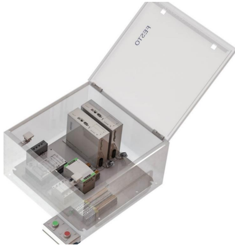
Figure 6-2. Design of the Electric Box.
